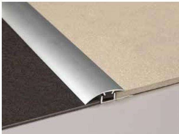
Patented end profile to join level differences from 0 to 6 mm. A plastic clip allows the elements of system MULTICLIP to be perfectly combined, creating a resistant and flexible system. The slight rotation of the finishing profile allows the system to seamlessly adapt to level differences.
